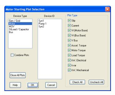
The Motor Acceleration Analysis module of ETAP is an excellent tool to simulate and investigate motor acceleration scenarios.
