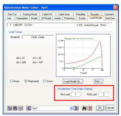
The data you have just seen and changed is the minimum necessary to run a simple Static Motor Starting study. Run the study by clicking on the Run Static Motor Starting button on the Motor Starting toolbar.
