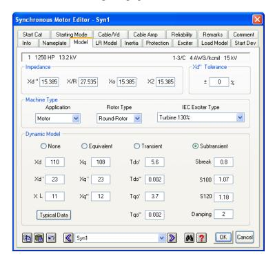
Now go to the Load Model page to view the load model. Ensure that a Load Model is entered for this motor. If a Load Model needs to be entered, click the Load Model Lib button, and accept a Motor Load by clicking OK in the window that appears.
